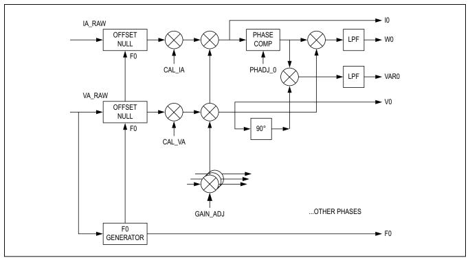
Figure 18. CE Data Flow—Offset, Gain, and Phase Compensation
