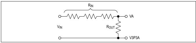
Figure 7. Typical Voltage Sense Circuit Using Resistive Divider
