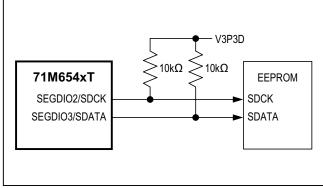
Figure 13. Typical I<sup>2</sup>C Operating Circuit
