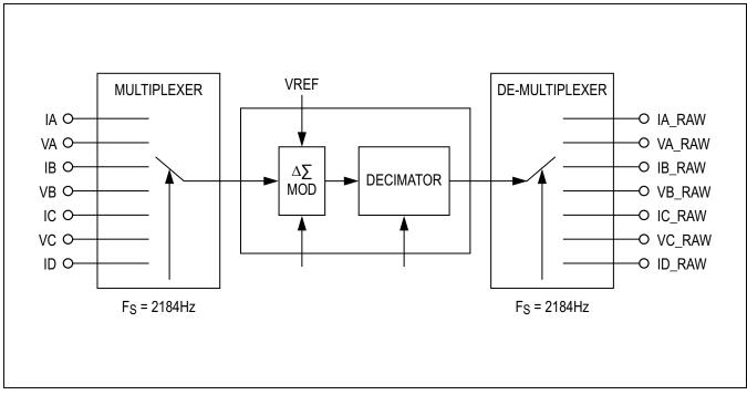
Figure 17. CE Data Flow—Multiplexer and ADC
