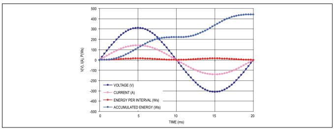
Figure 6. Waveforms Comparing Voltage, Current, Energy per Interval, and Accumulated Energy
