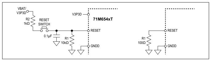
Figure 15. Typical Reset Circuits
