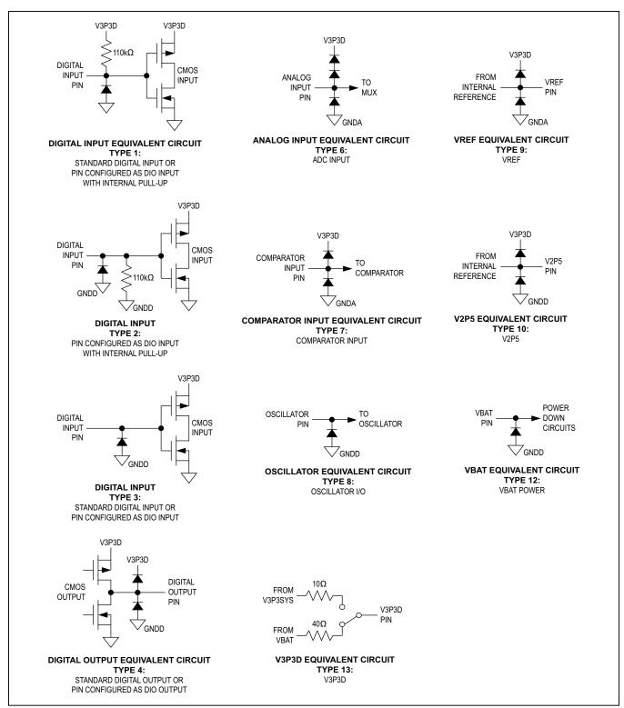
Figure 1. I/O Equivalent Circuits
