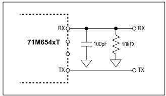
Figure 14. Typical UART Operating Circuit
