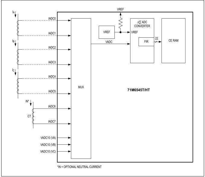
Figure 2. 71M6545T/HT Operating with Local Sensors
