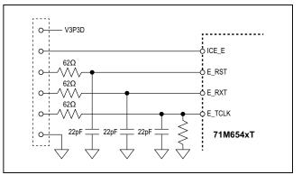
Figure 16. Typical Emulator Connections
