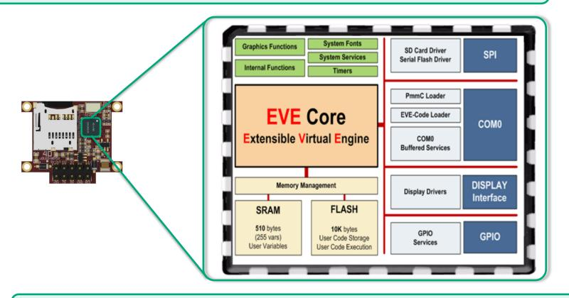
The GOLDELOX offers a complete suite of features, crafted to be at the forefront of any product requiring colour, animation, images and sound. The GOLDELOX is also powerful enough to control and communicate with peripheral devices over SPI, One Wire or Serial Port.
