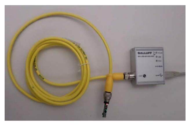
Figure 1. Santa Cruz Board Connected to a Balluff USB IO-Link Master
