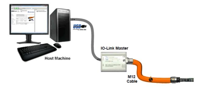
Figure 3. Block Diagram of System
