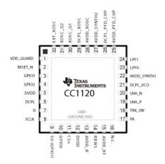
The device is mainly intended for Industrial, Scientific, and Medical (ISM) applications and Short Range Device (SRD).
