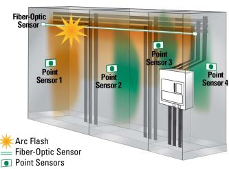
Scenario with point sensor placement on the wall of each compartment. Arc detection area for each sensor is shown in green shade. In this case, both Point Sensor 1 and the Fiber-Optic Sensor detected the flash as it was within their viewing area (shown in orange).
