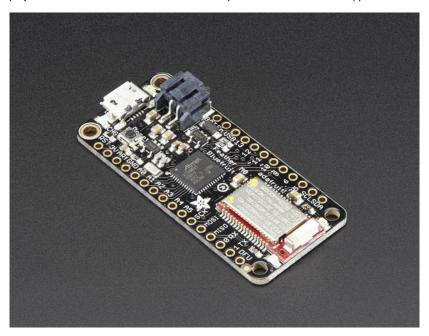
At the Feather M0's heart is an ATSAMD21G18 ARM Cortex M0 processor, clocked at 48 MHz and at 3.3V logic, the same one used in the new <a href="Arduino Zero">Arduino Zero</a> (http://adafru.it/2843). This chip has a whopping 256K of FLASH (8x more than the Atmega328 or 32u4) and 32K of RAM (16x as much)! This chip comes with built in USB so it has USB-to-Serial program & debug capability built in with no need for an FTDI-like chip.
