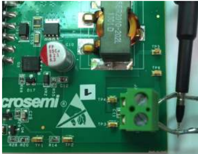
Figure 11. Proper ripple measurement
