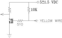
13-1. THE FAN SPEED WILL DEFAULT TO MAXIMUM WHEN THE SPEED CONTROLL INPUT IS LEFT UNCONNECTED.
