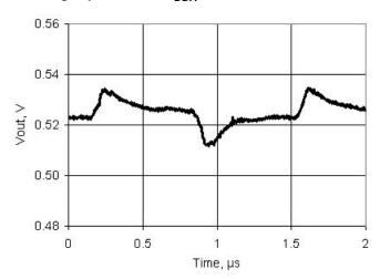
Figure 11-51. VDAC Voltage Noise, 1 V Mode, High speed mode,  $V_{\text{DDA}}$  = 5 V
