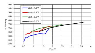
Figure 11-13. Efficiency vs  $V_{BAT}$ ,  $L_{BOOST}$  = 22  $\mu H$  [35]
