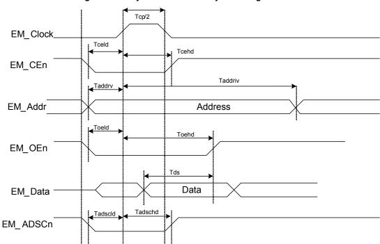
Figure 11-55. Synchronous Read Cycle Timing
