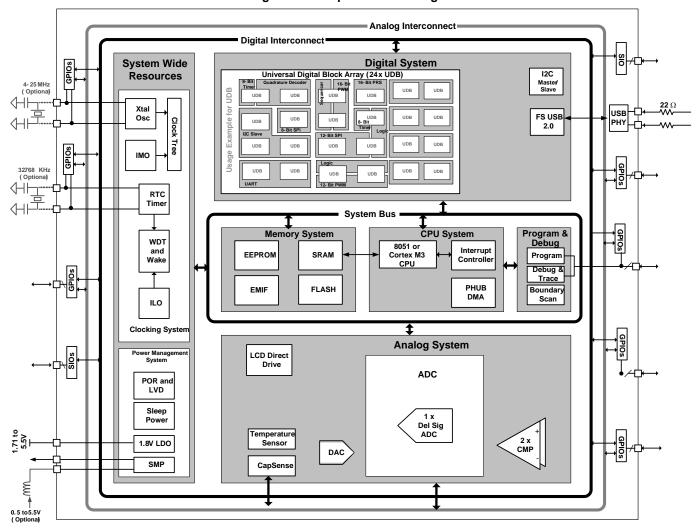
Figure 1-1. Simplified Block Diagram
