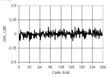
Figure 11-31. IDAC DNL vs Temperature, Range = 255  $\mu\text{A}$ , High speed mode
