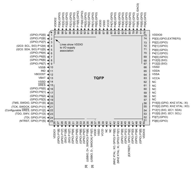
Figure 2-6. 100-pin TQFP Part Pinout
