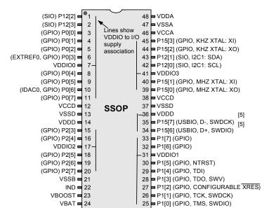
Figure 2-3. 48-pin SSOP Part Pinout
