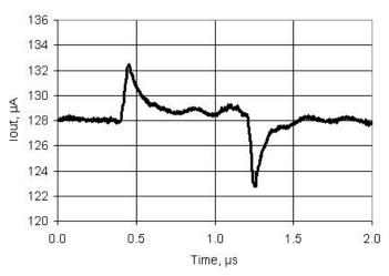
Figure 11-39. IDAC Current Noise, 255  $\mu$ A Mode, Source Mode, High speed mode, V<sub>DDA</sub> = 5 V
