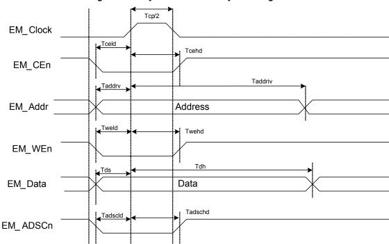
Figure 11-56. Synchronous Write Cycle Timing
