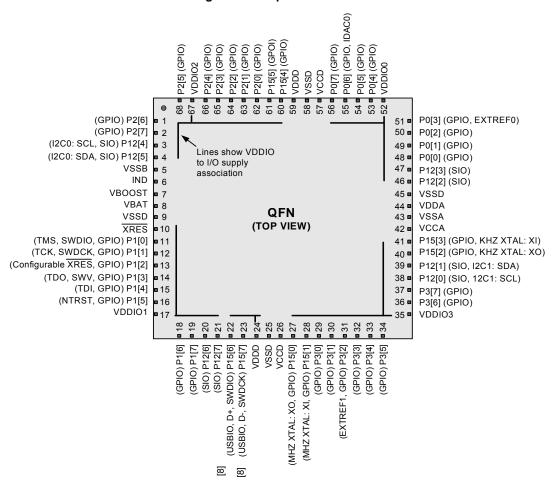
Figure 2-5. 68-pin QFN Part Pinout<sup>[7]</sup>
