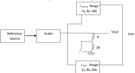
Figure 8-7. DAC Block Diagram
