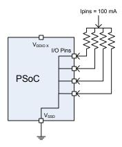
For the 48-pin devices, the set of I/O pins associated with VDDIO0 plus VDDIO2 may sink up to 100 mA total. The set of I/O pins associated with VDDIO1 plus VDDIO3 may sink up to a total of 100 mA.
