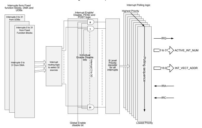
Figure 4-3. Interrupt Structure
