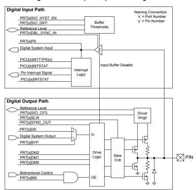
Figure 6-10. SIO Input/Output Block Diagram
