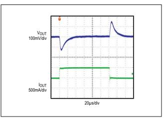
Figure 5. MAX17502F 500mA to 1A Load Transient
