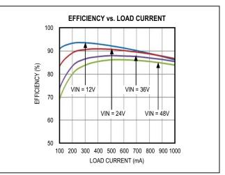
Figure 2. MAX17502F Efficiency
