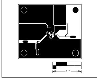
Figure 8. MAX17502F EV PCB Layout—Component Side
