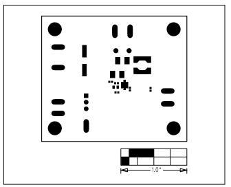
Figure 10. MAX17502F EV Kit PCB Layout—Top Solder Mask
