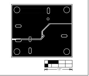
Figure 9. MAX17502F EV Kit PCB Layout—Solder Side
