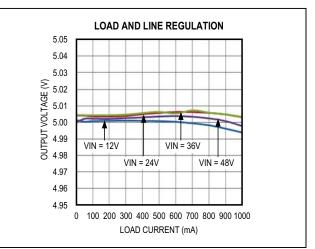
Figure 1. MAX17502F Load and Line Regulation
