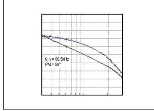
Figure 3. MAX17502F Full Load Bode Plot (VIN = 24V)
